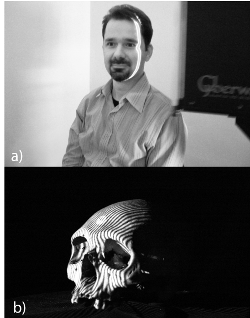
Fig. 2 - Laser – versus fringe projection scanner. Scanners using a class 1 or 2 laser are considered eye-safe and can be used on live subjects. The Colour version is available online at JASs web site.
